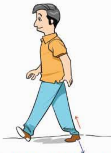
Fig. 10.03 : At the time of walking, when a man pushes the ground with feet, ground also pushes him equally.
