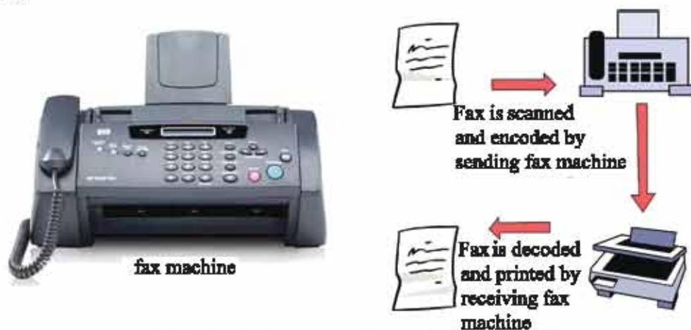
Fig. 13.12: Fax machine and its functioning
