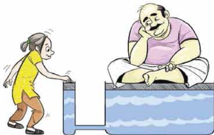
Figure: 5.16 : A man is lifted up by putting pressure on a hydraulic press
