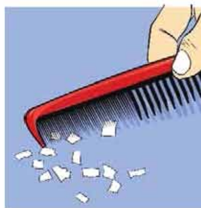
Figure 10.05: During winter, combing hair and the comb is held near the pieces of paper, they feel attraction.
