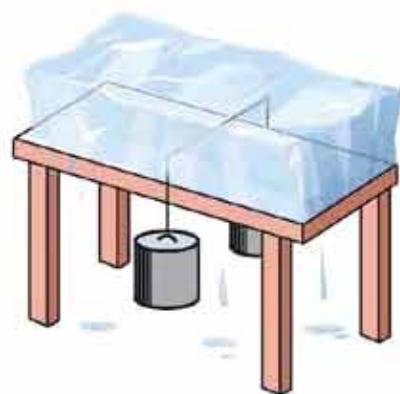
Figure 6.09: It is possible to cut a ice bar by pressing with a fine wire.
