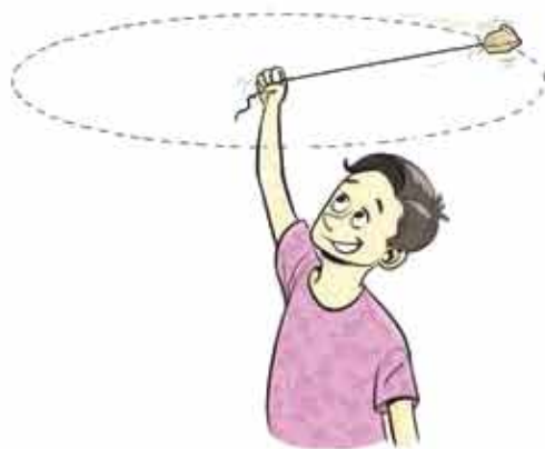
Figure 2.05 : In case of rotation of a stone tied with string, velocity might be changed though speed is same.
