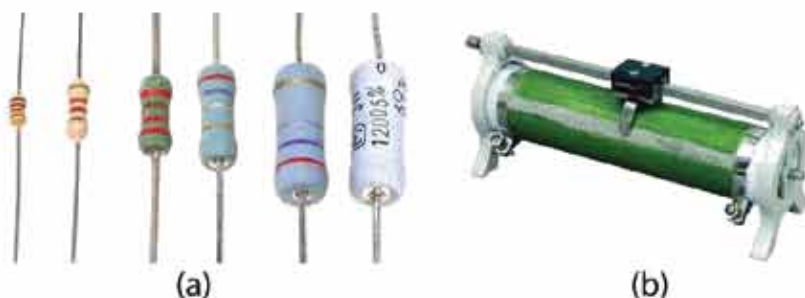
Figure 11.06: (a) Fixed and (b) variable resistors
