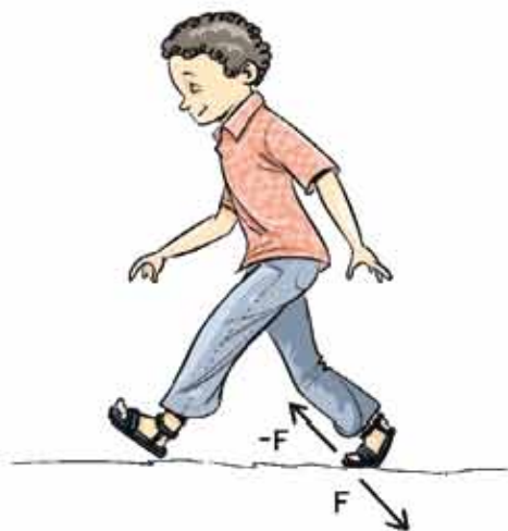
Figure 3.13: During walking when a person applies force on the ground then the ground also applies force on him in contrary
