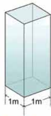
Figure 5.06: The pressure of air comes from the weight of the air column.
