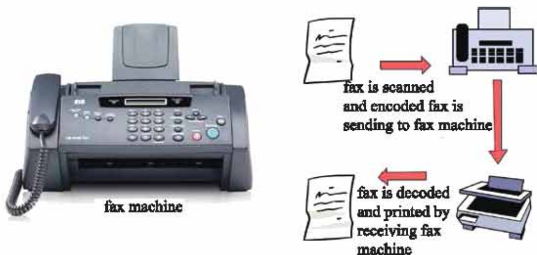
Figure 13.17: Fax machine and its functioning.
